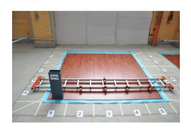
the 100 kg load were applied to the flooring surface in sector A1 (LOAD ON position) and readings were taken from all 5 micrometers wich were positioned in sectors: A1, A2, A3, A4, A5
