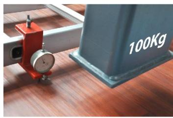
100 kg load was removed from the flooring surface in sector A1 (LOAD OFF position) and readings were taken from all 5 micrometers
