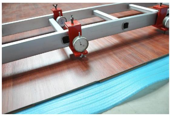
Vertical movement of the laminate flooring in a combination with different underlays under dynamic load (a simulated walking)
