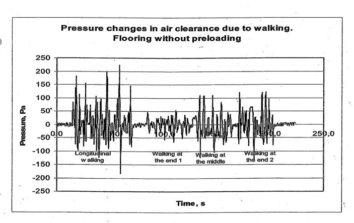
Figure 1. Pressure changes in air clearance due to walking. Flooring without preloading.
